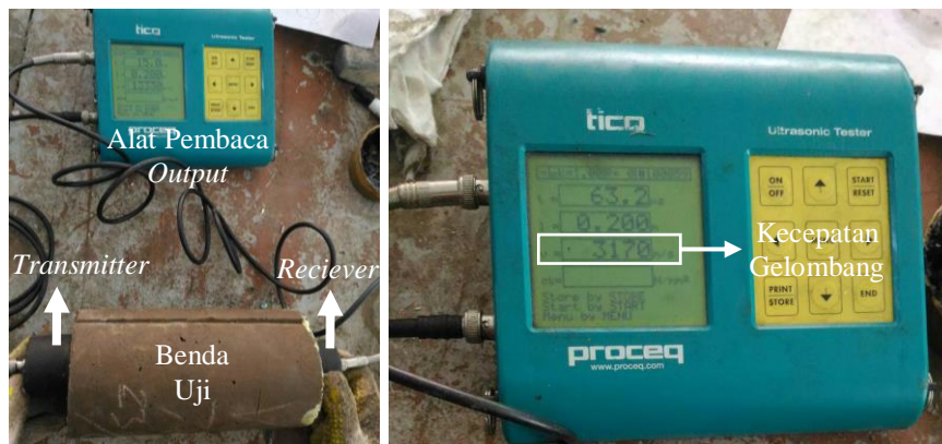
Gambar 6. Pengujian UPV ( Ultraviolet Pulse Velocity )
