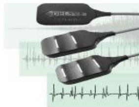
Gambar 2.4 Surface EMG Sensor (Mehrkanoon, Saeid. 2008)
